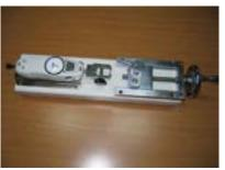
Wire & crimped terminal tensile tester
