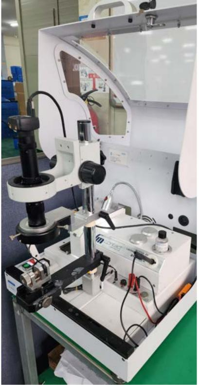
Cross section camera for crimped terminal
