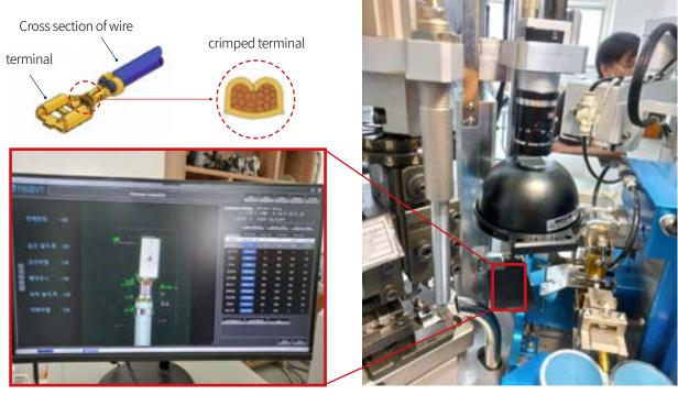
Real-time crimped form, size monitoring, and MES linkage
